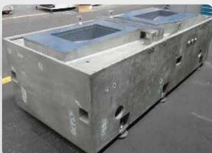
Fabricated Bed with Anti-Friction Concrete for HIGH RIGIDITY
