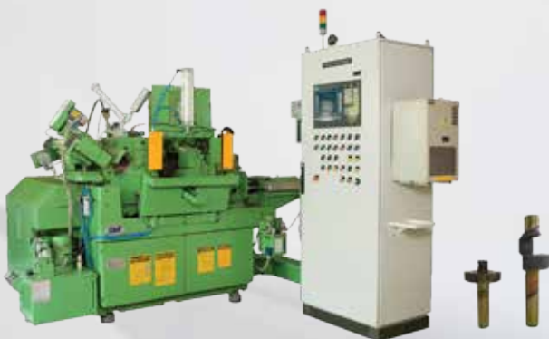
SMT NO.2-10" 3 AXIS CNC GRINDER FOR CRANKSHAFTS. AUTO LOADER AND LIGHT SENSITIVE CURTAINS
