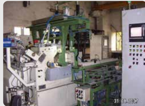
SMT NO.2-10" WITH 3 AXIS CNC TOOLED UP FOR GRINDING HYDRAULIC SPOOLS. ALSO EQUIPPED WITH AUTO LOADER, AUTO BALANCER
