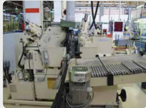
SMT NO.2-10" CONVENTIONAL GRINDER TOOLED UP FOR THRUFEED GRINDING OF SHOCK ABSORBER SHAFT
