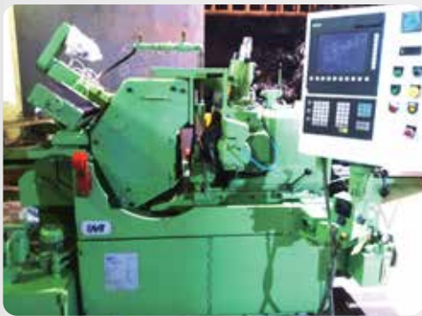
SMT NO.2-10" WITH 3 AXIS CNC FOR GRINDING ENGINE LINERS
