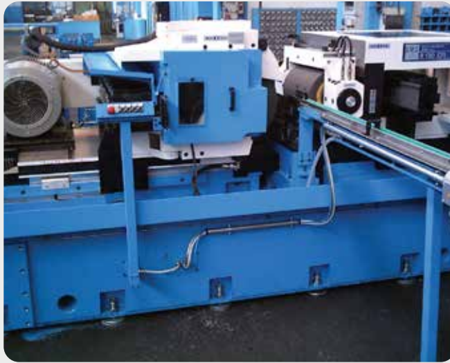
R50 BMS-SMT TOOLED UP FOR ROUGH AND FINISH GRINDING OF TEXTILE SPINDLE
