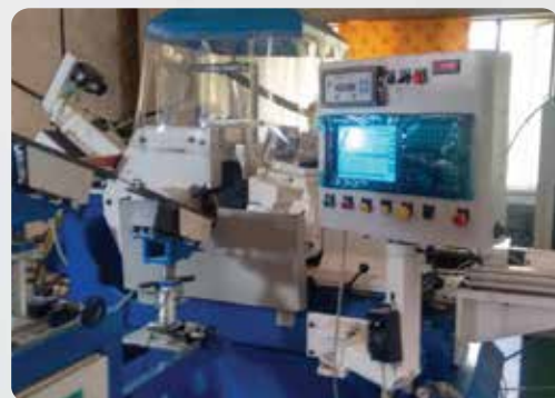
SMT NO.2-10" WITH 3 AXIS FOR GRINDING PINS OF Ø 2mm 3 AXIS CNC WITH BOWL FEEDER
