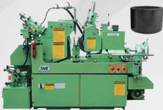
SOLAIRE NO.2-8" CONVENTIONAL GRINDER TOOLED UP FOR THRUFEED GRINDING OF CERAMIC COMPONENTS
